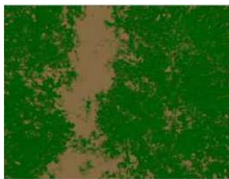
Fig. 2a: Straight down image of Tajikistan grassland (before). Fig. 2b: Processed image using VegMeasure software (after): plant cover 78.5%, bare ground 21.5%, classification accuracy: 98%
